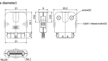
• 36 pos. (Shielded type, for 7mm max. cable diameter)
