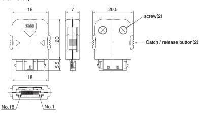
18 pos. (Reverse, shielded type, for 4mm max. cable diameter)
